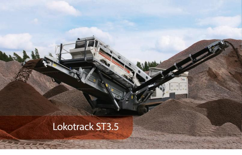
The Lokotrack® ST3.5™ is designed with compact transport dimensions, high-quality components, and to meet the latest global health and safety legislation. The standard ST3.5 two-deck Lokotrack is capable of producing two-sized fractions, and depending on the application, an optional two-deck vibrating grid can be installed to yield fractions of three sizes.
