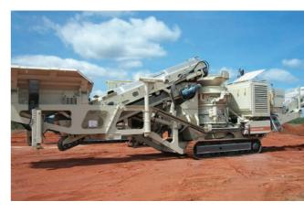
Lokotrack LT300HP is available with either a belt feeder or alternatively with a vibrating grizzly feeder.
